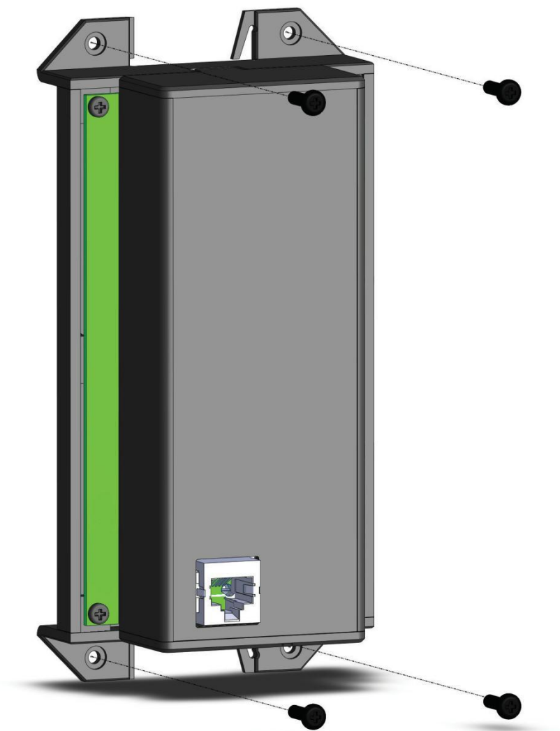
Figure 2 - Wall Mounting with Screws
